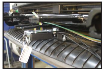
14. **Optional Breakaway:** Attach the bracket to the lower valance with the 1/4" hardware at the desired location. Attach the breakaway to the bracket with the supplied 1/4" hardware.
