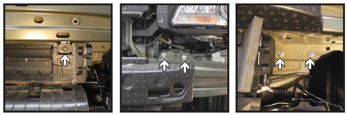
Using a 10MM socket, remove the two (2) screws from the shutter system underneath the bumper (left). There is one (1) on each side.
