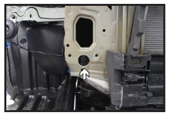
8. Using a 1-1/4" hole saw, drill an access hole on the passenger side only.
