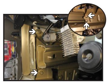
5. Using a 14MM socket, remove the four (4) bolts from the brace on the driver side and set aside.
