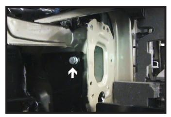
Using a 3/8" drill bit, drill the top front hole on the passenger side thru the frame. Install the 3/8" hardware into the hole with a 3/8" nut plate on the inside of the frame. Fully tighten the bolt.
