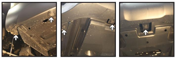
3. Remove the nine (9) push pins from the underside of the fascia. There are four (4) on each side and one (1) in the middle.
