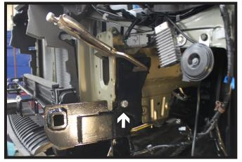
9. Position the baseplate onto the frame. On the driver side, start the 10MM bolt/lock washer into the existing hole with the DS spacer tube in between the baseplate and frame. Level and clamp the baseplate into position. Fully tighten the 10MM bolt on the driver side.
