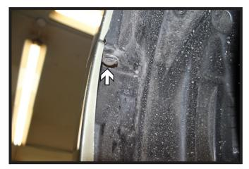
2. Remove the push pin in the wheel well along the fascia/fender joint. Do this on both sides of the vehicle.
