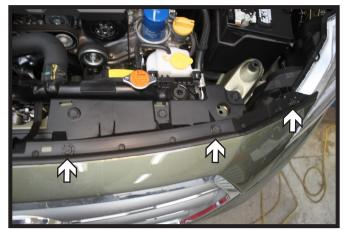
1. Remove the six (6) push pins from the top of the fascia. There are three (3) on each side.
