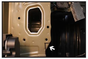
7. Using a reciprocating saw, trim a notch on the driver side only for baseplate clearance.
