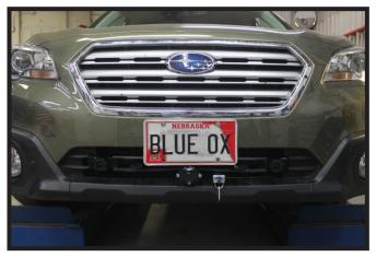
15. Hold the fascia as close to its original position, mark and trim the fascia around the convenience links and attachment tabs. Reinstall the fascia.
