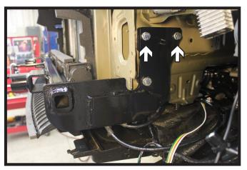
11. Using a 3/8" drill bit, continue drilling the remaining holes on the baseplate thru the frame. Install the 3/8" hardware into the remaining top holes with 3/8" nut plates on the inside of the frame (white).
