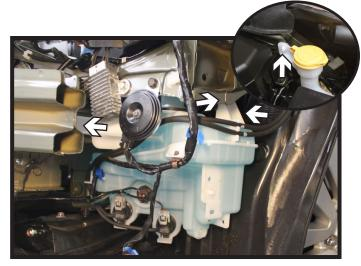
Unsnap the reservoir neck from the firewall (inset). Using a 10MM socket, remove the two (2) screws and one (1) nut from the washer reservoir. Disconnect/ plug all lines and set the reservoir aside.
