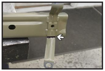
13. On the driver side brace, trim off the lower arm and reinstall the brace to the vehicle.Reinstall the bumper & washer reservoir.
